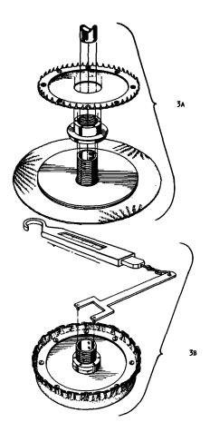
FIG. 3—Illustration showing attachment of fabric specimen to an abrasion pad; (a) before attaching fabric over hooks and (b) during torquing of fabric.
