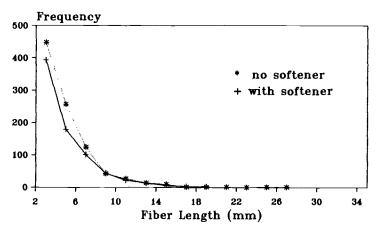
FIG. 7—Length distribution of fibers  $\geq 2 \text{ mm transferred}$ —woven MSL fabrics (A, B, C, and D).
