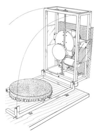
FIG. 2—Illustration of the FTAT swung open and resting in the upright position.
