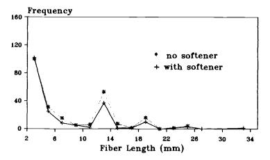
FIG. 8—Length distribution of fibers  $\geq 2$  mm transferred—knit MSL fabrics (G and H).
