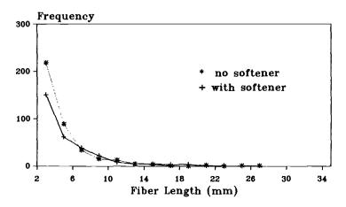
FIG. 5—Length distribution of fibers  $\geq 2 \text{ mm transferred}$ —non-MSL fabrics (E, F, and I).
